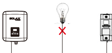
Incorrect Connection between Load and Inverter
