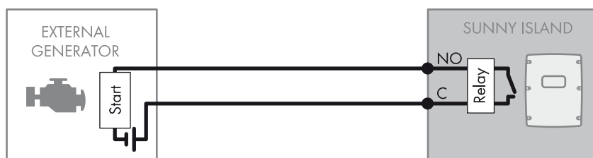
Figure 15: Connection of the generator control to the Sunny Island
