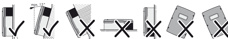
Figure 5: Permissible and impermissible mounting positions
