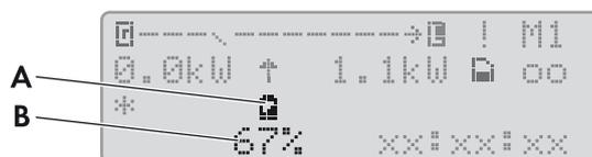
Figure 10: State of charge of the battery in standard mode (example)
