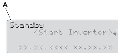
Figure 4: Display of operating states (example **Standby**)
