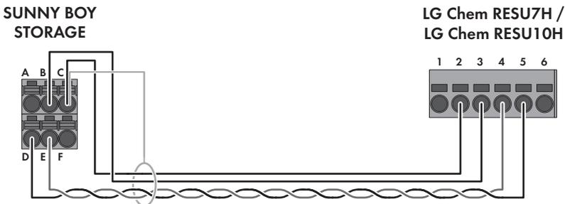
Figure 1: Cabling plan SBS2.5-1VL-10 with RESU7H / RESU10H
