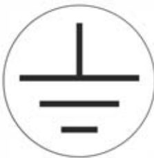
Figure 2.18 Grounding conductor symbol
