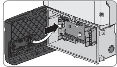
2. Ensure that the ribbon cable is securely plugged into the sockets at both ends.
