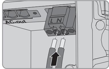
13. Ensure the conductors are plugged into the terminal points (round openings) as far as it will go and not into the actuation shafts (rectangular openings).
