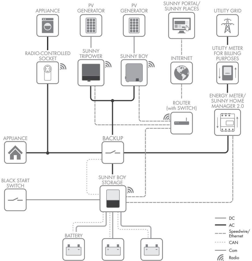
Figure 4: System design of a flexible storage system with battery-backup function (example)
