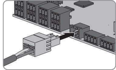
7. Ensure that the terminal block is securely in place.
