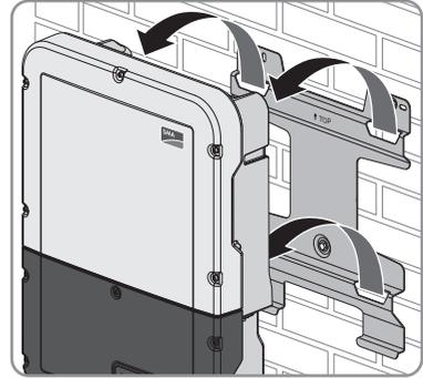
16. Unscrew the screws for fastening the wall mounting bracket and remove the wall mounting bracket.
