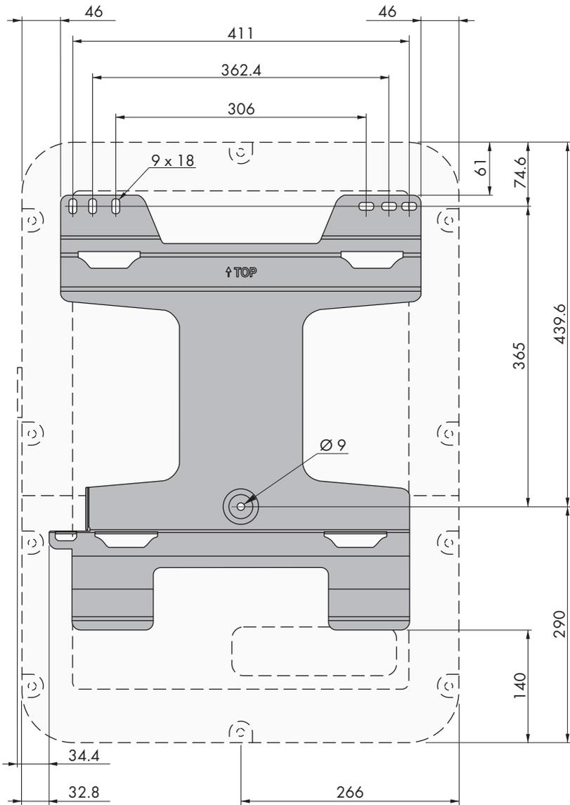
Figure 7: Position of the anchoring points(Dimensions in mm)
