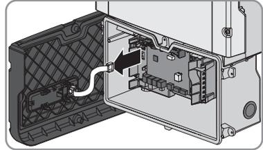
6. Ensure that no voltage is present on the **AC-out** terminal block between **L** and **N** using a suitable measuring device. To do this, stick the test probe in each rectangular opening of the terminal.
