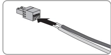
6. Stick the terminal block into the slot
