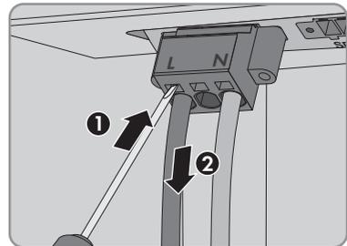
4. Screw out the screws from the **AC-out** terminal block using a flat-blade screwdriver (blade width: 3.5 mm) and pull the terminal block out of the slot.
