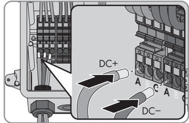
8. Ensure that the terminal points are allocated to the correct conductors.
