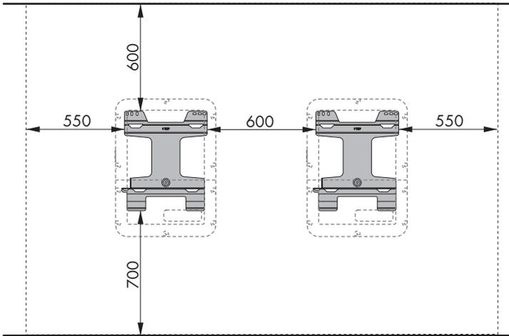
Figure 8: Recommended clearances(Dimensions in mm)
