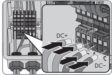
7. If there is only one battery that is rated for a maximum charge/discharge current of the inverter of 10 A, connect the cables to input A. Insert each conductor into the corresponding terminal point.
