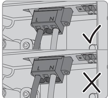
16. Ensure that the terminal points are allocated to the correct conductors.
