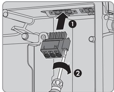
8. Ensure that the terminal block is securely in place and the screws are tightened.
