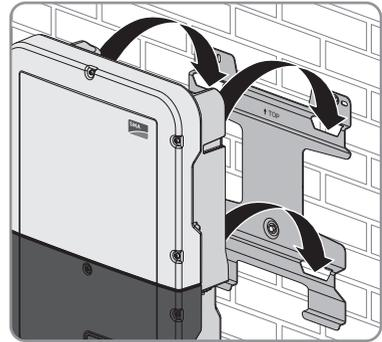
7. Check whether the inverter is securely in place.
