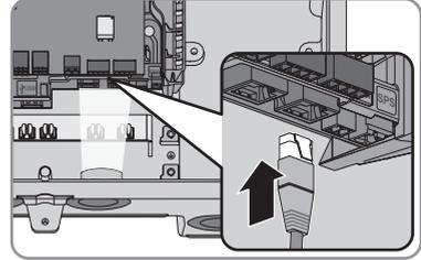
9. Ensure that the network connector is securely in place by pulling slightly on each cable.
