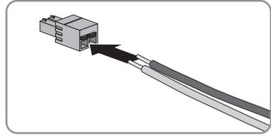
6. Stick the terminal block into the slot
