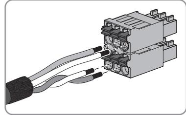
9. Make sure that the conductors are plugged into the terminal points tightly by pulling slightly on the conductors.
