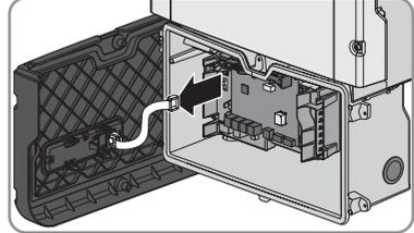
3. Remove the adhesive tape from the enclosure opening for the AC connection.
