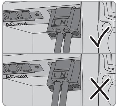
14. Ensure that the terminal points are allocated to the correct conductors.
