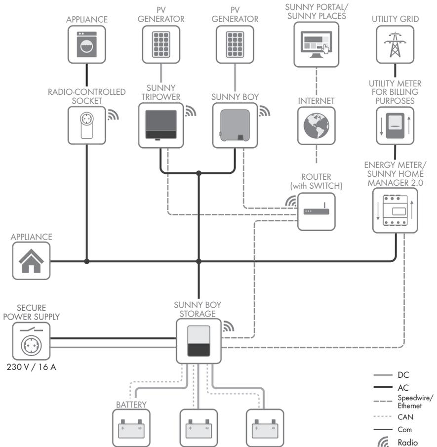
Figure 3: System design of a flexible storage system with switch and outlet for secure power supply operation (example)
