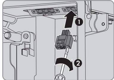
7. Ensure that the terminal block is securely in place.
