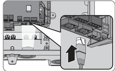
10. Ensure that the network connector is securely in place by pulling slightly on each cable.
