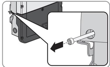
15. Remove the inverter by lifting it vertically up and off the wall mounting bracket.
