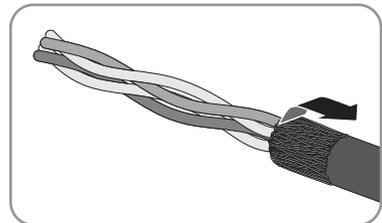
6. Strip the insulation on the insulated conductors each by 6 mm. The **CAN L** and **CAN H** must be a twisted pair.
