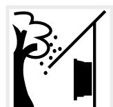
Protect inverter from falling parts which could enter the inverter's ventilation openings.
