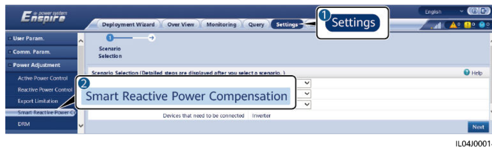
Figure 6-53 Setting parameters for smart reactive power compensation
