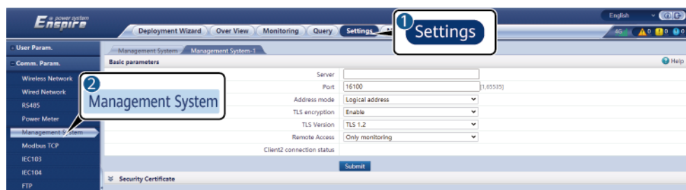
Figure 6-10 Setting management system-1 parameters
