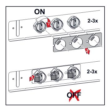
With the DC disconnector lock, the inverter can be secured against unintentional switching off.
