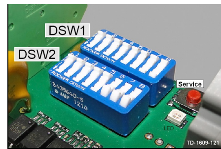
Position of the DIP-switches DSW1/2
