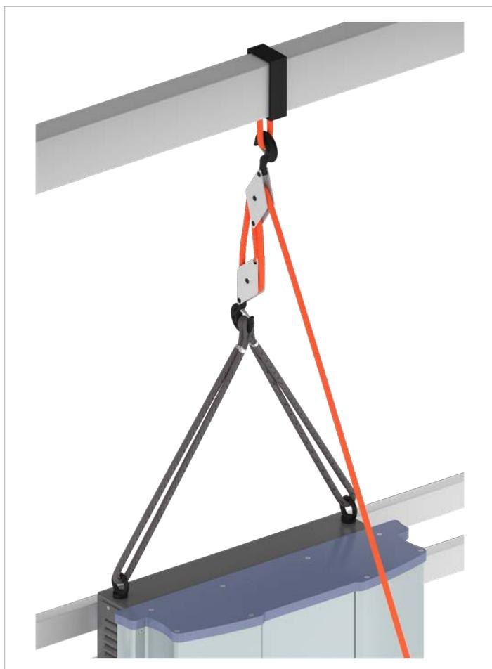
16. Secure the inverter with a block and tackle or with crane so that the weight will be suspended from the block and tackle after the mounting screws are loosened.
