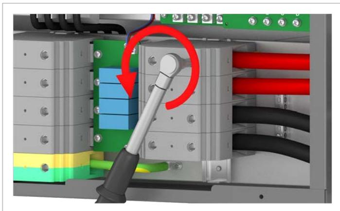
5. Unscrew the DC cables on the DC terminal block.
