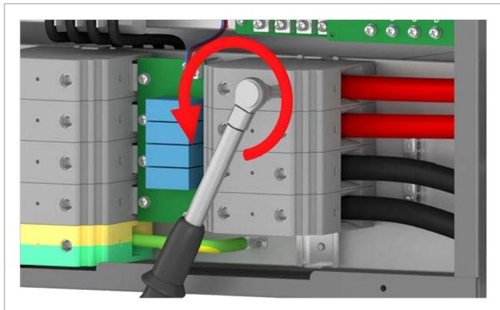
5. Unscrew the DC cables on the DC terminal block.
