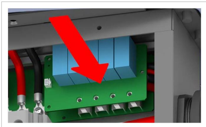
4. Fit the new block with the surge protection devices and screw in place using the 5 screws.
