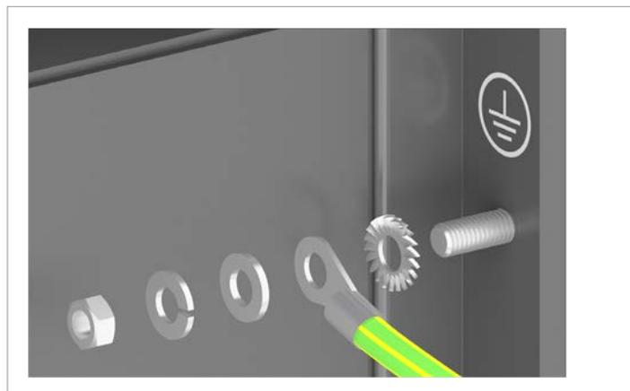
2. Perform a continuity check of the grounding connection. If there is insufficient conductive connection, scratch away the paint from the inverter housing under the toothed lock washer to achieve a better electrical contact.
