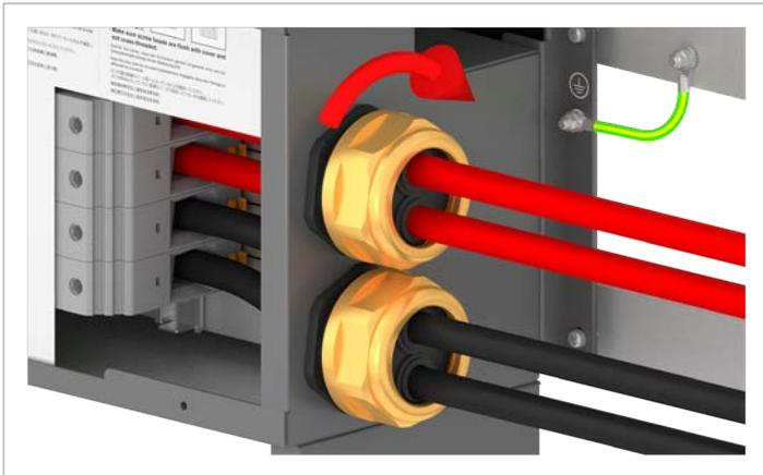
7. Secure the DC cables with a strain relief element.
