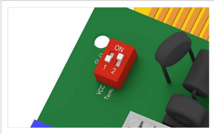
2. Set the DIP switch for the RS485 termination resistor (DIP 2) to the **ON** position.
