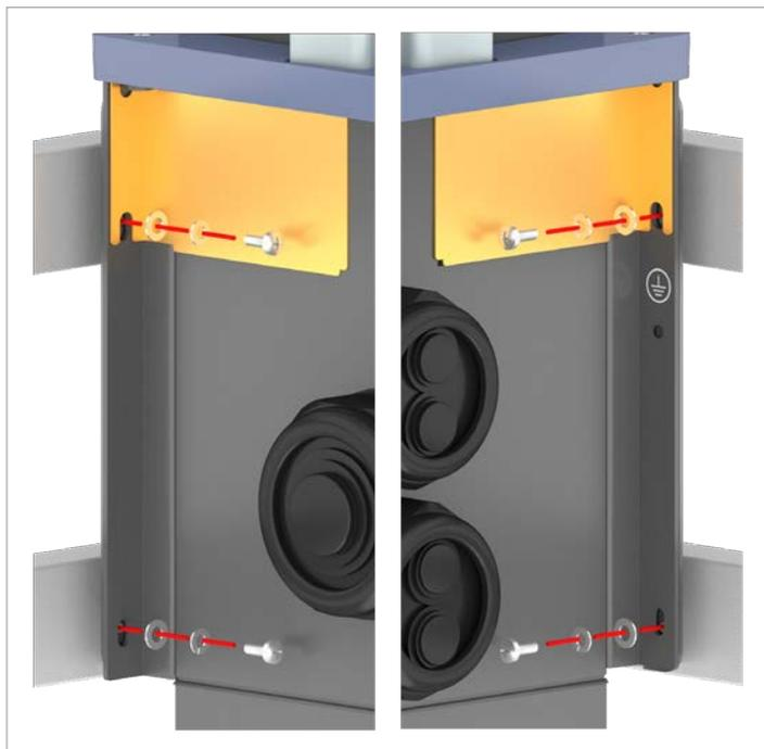
5. If desired, mount the cover panels for the side air inlets.
