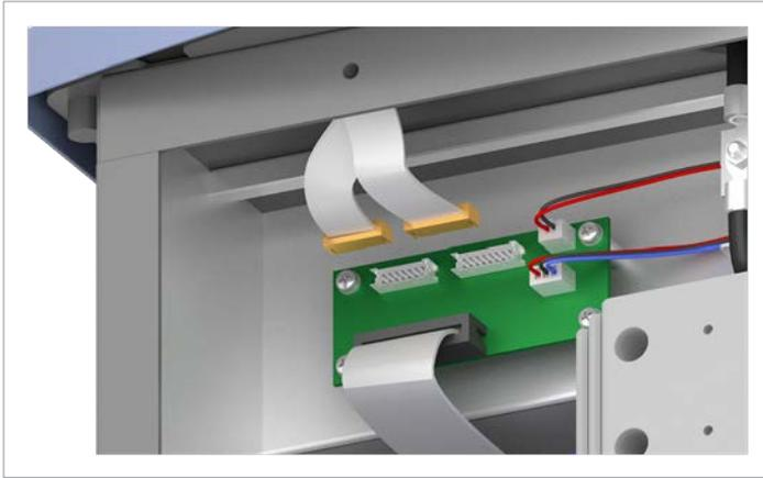
10. At the top left circuit board, plug in the two upper plugs with the internal communications cables.
