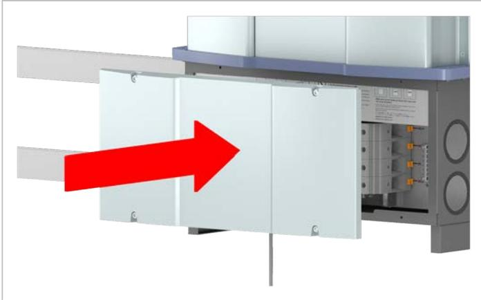
12. Fit the terminal box cover and screw it into place.
