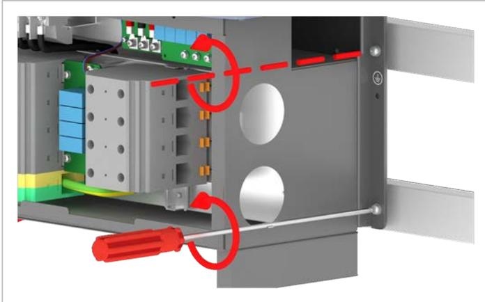
17. Unscrew the junction box from the mounting plate.
