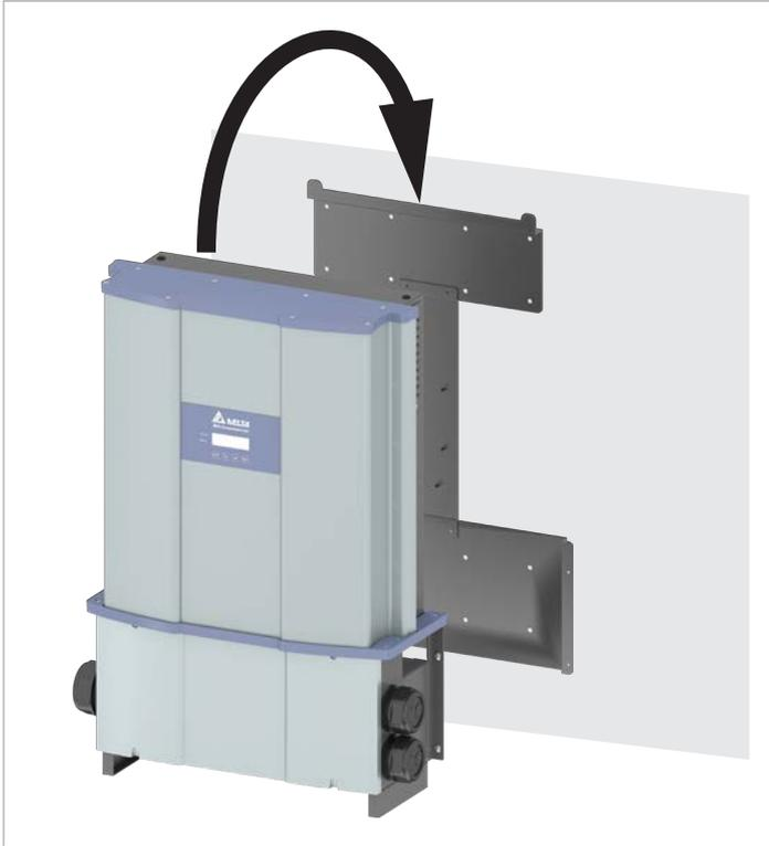
2. Mount the inverter on the mounting plate.
