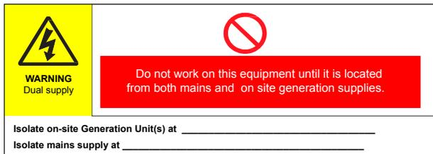
13. In accordance with local regulations attach warning labels to the outside of the inverter as necessary.
