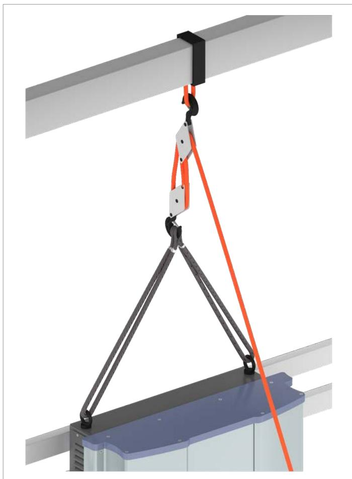
14. Secure the inverter with a block and tackle or with crane so that the weight will be suspended from the block and tackle after the mounting screws are loosened.
