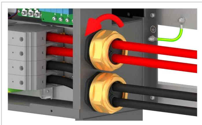
6. Unscrew the DC cable gland and carefully pull out the DC cables.
