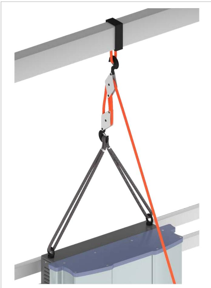
9. Secure the inverter with a block and tackle or with crane so that the weight will be suspended from the block and tackle after the connection screws to the junction box have been loosened.
