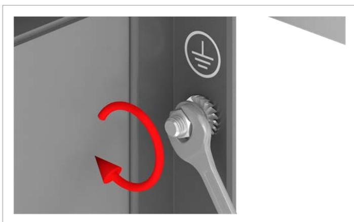
14. Screw the ground screw back on.
