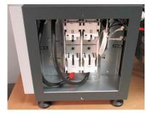
4. Remove cable tie from the USB cable. Remove the USB plug form the rear wall.
