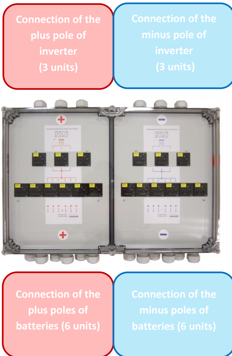
Figure 4-16: BAT BREAKER Box of Enwitec (example for 6 batteries and 3 inverters) with a closed housing
