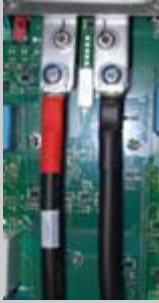
Figure 4-5: sample representation of the connection of plus and minus power cables with the SMA Sunny Island inverter
