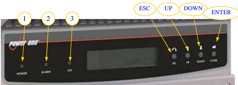
Fig. 20 - Location of buttons and LEDs
