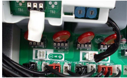
Fig. 14B - Positive grounding
