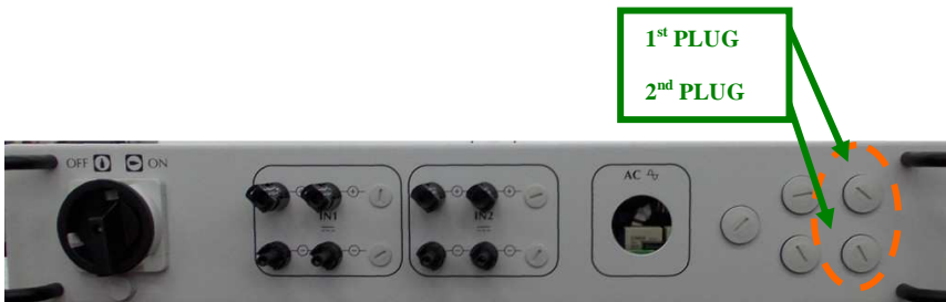
Fig. 24 - Cable routing for RS-485 connection
