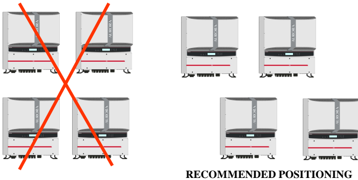
Fig. 5 - Recommended installation of AURORA inverters
