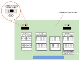
Fig. 6-6 Communication configuration
