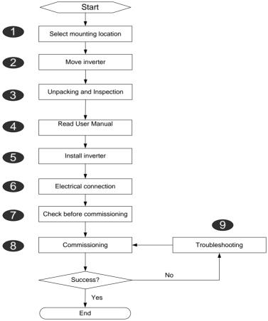
Fig. 3-1 Installation flowchart
