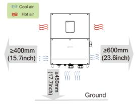
When installing multiple inverters, it is recommended to install multiple devices side by side.
