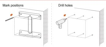
Step 5 Secure the bracket to the wall firmly by the supplied expansion bolt sets.
