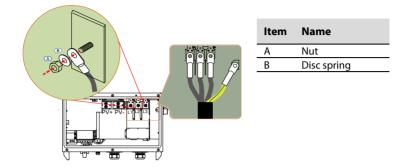
recommended tightening torque range is 34~40 N·m.
