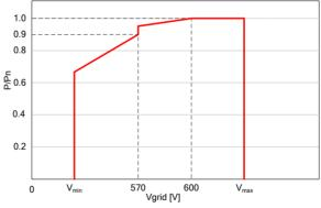
Fig. 2-7 Grid under-voltage derating(Pf=1)
