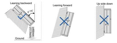
• If the included angle between the installation site and the plumb line is greater than 75°, install the inverter on the frame to meet the requirement for installation angle. The frame and the inverter are installed as shown in the following figure.
