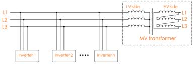
Fig. 6-2 Multiple Inverters in parallel Connection
