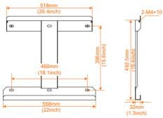
Fig. 5-1 Dimensions of the bracket (figures in inch)
