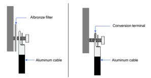
Beware the direction of the albronze filter, i.e. the copper side must be closely attached to the copper bar and the aluminum side must be closely attached to the aluminum connection terminal.
