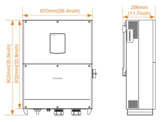
Fig. 2-3 Dimensions of the inverter
