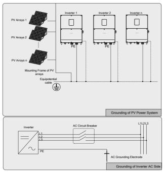
Fig. 6-3 Grounding of inverter
