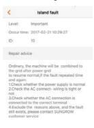
Fig. 10-11 Detailed fault alarm info
