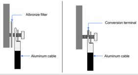
Beware the direction of the albronze filter, i.e. the copper side must be closely attached to the copper bar and the aluminum side must be closely attached to the aluminum connection terminal.
