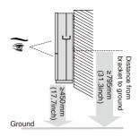
Install the inverter vertically or at a maximum back tilt of 75 degrees. Do not
