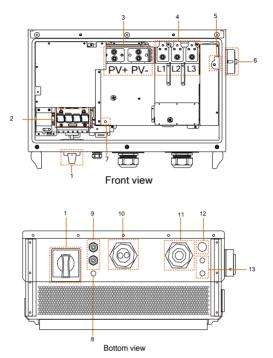
Fig. 6-1 Cable connection area
