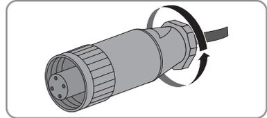
13. When using the cable gland, screw the cable gland firmly onto the threaded sleeve.
