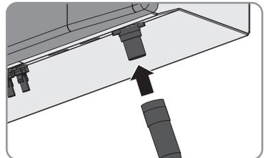
15. If the AC connection socket is not to be connected to the inverter immediately, close the AC pin connector on the inverter with the protective cap provided.
