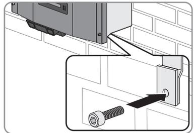
9. Ensure that the inverter is securely in place.
