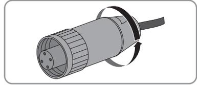
12. When using pressure screw, fastening case and sealing ring, screw the pressure screw firmly onto the threaded sleeve. The fastening case will be pressed into the threaded sleeve and no longer be visible.
