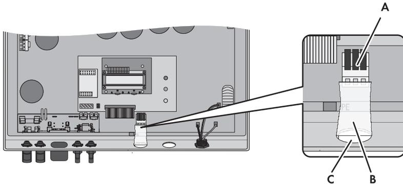
Figure 10: Position of the fault indicator relay and cable route
