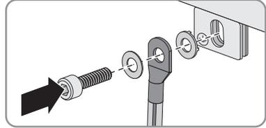
4. Insert the cylindrical screw through the metal shackle on the inverter and screw it onto the wall mounting bracket (torque: 6 Nm).
