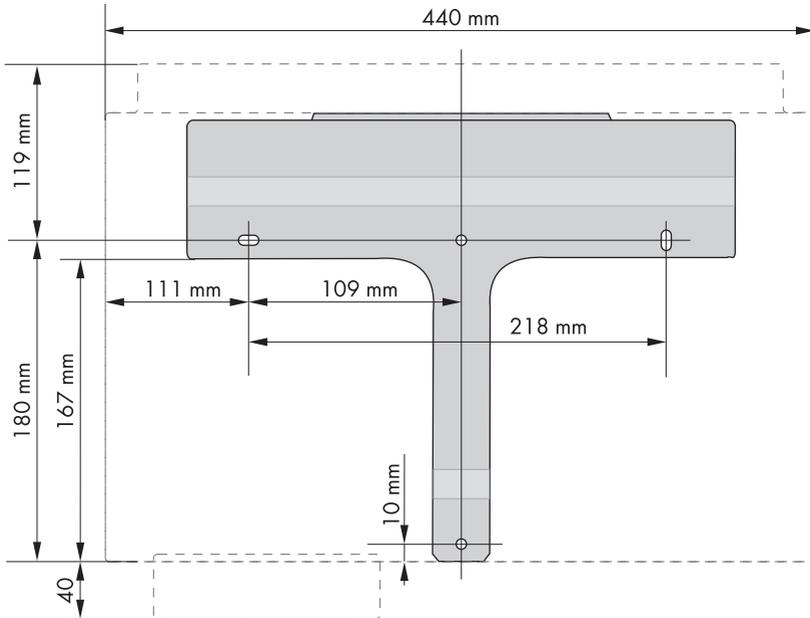
Figure 3: Wall mounting bracket dimensions
