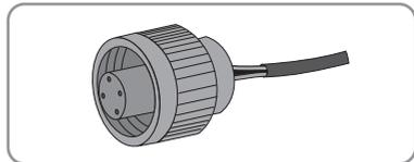
11. Screw the threaded sleeve tightly onto the bush insert.
