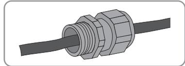
8. Slide the threaded sleeve over the AC cable.
