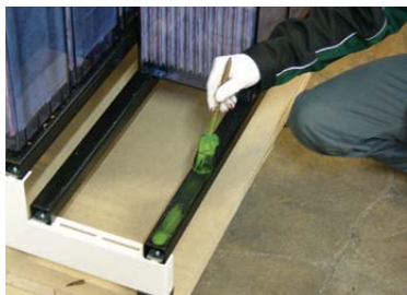
Fig. 5-13: Greased support profiles
